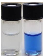
Figure 7. Methyl viologen before (left) and after photocatalytic reduction (right). General conditions: 50 mM Tris-HCl buffer (pH 8); [EDTA] = 10 mM; [dRf] = 20 \mu M; [MV] = 20 \mu M; T = 25 ^{\circ} C; \lambda = 450 nm; anaerobic.
