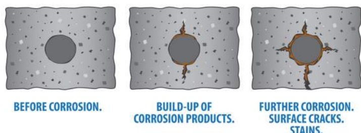
Figure 10.1: Development of corrosion cracking (The helpfull engineer, 2010)
