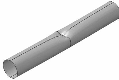
Figure 6.4 Maximum deformed tube for internal pressure level of  $q=0.4$ . Localization of denting is observed.
