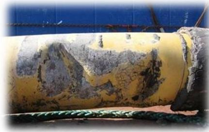
Figure 2.1 Dented pipe after removal operation. (Karamanos, Pournara, 2013)
