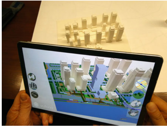
Fig. 1.10 Mobile tablet-based AR by implementing with 3D model recognition and tracking with for superimposing designs of blue and green infrastructure and virtual replacement of buildings in the physical model. Photo Eckart Lange
