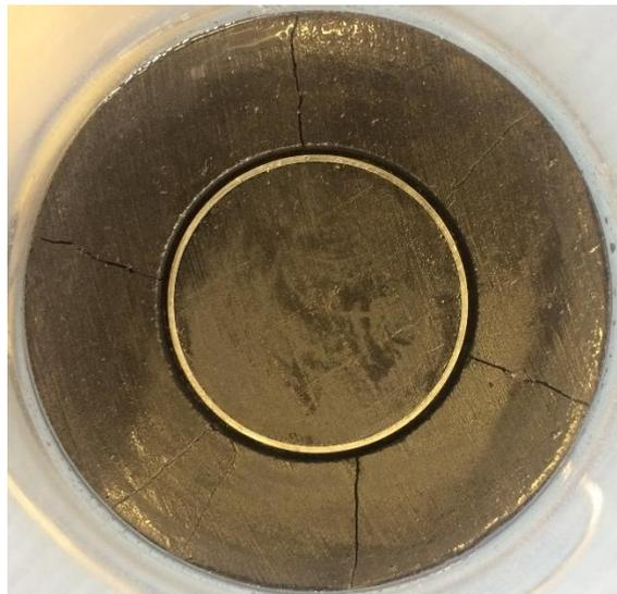
Figure 7.10: Top view of the CKO6-AA-01-02-02s after the PTS test showing a set of radial fractures which initiated during the hydrostatic unloading of the sample.
