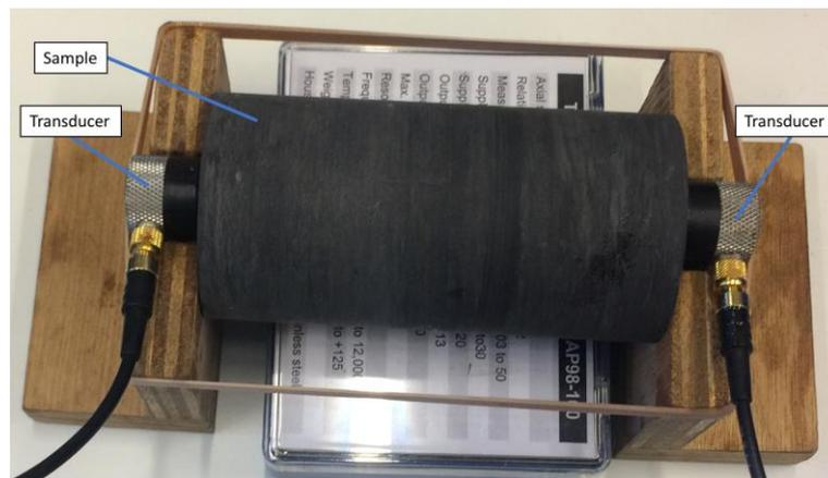
Figure 3.6: Overview of the setup during ultrasonic p- and s-wave measurements.
