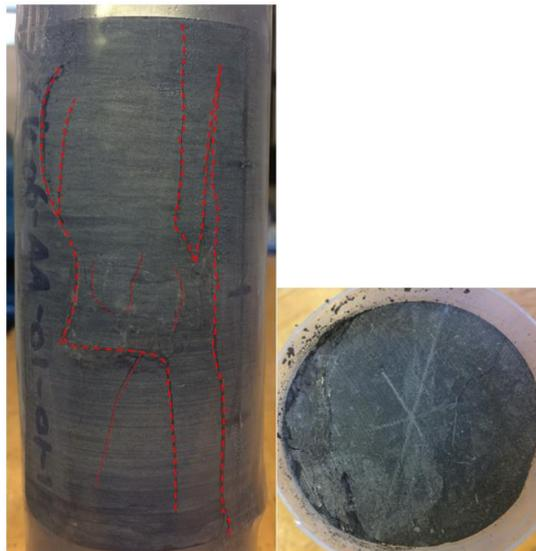
Figure 5.8: CKO6-AA-01-01-11s rock sample after uniaxial compression test.
