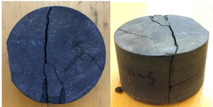
Figure 5.5: CK06-AA-01-02-11s after Brazilian testing showing non tensile failure
