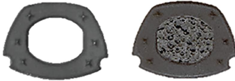
**Figure 8-3:** Cervical cages in  $\text{Si}_3\text{N}_4$  used for the study by Suh et al. [17]. On the left, the cage with an empty core; on the right, the cage core is filled with load-bearing porous  $\text{Si}_3\text{N}_4$ .
