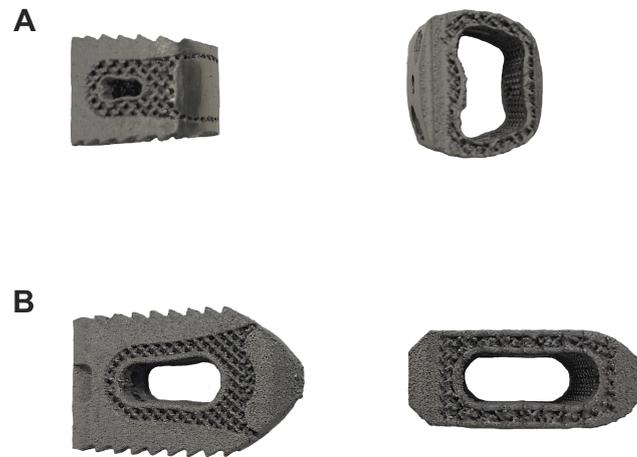
**Figure 5-4:** Cervical (A) and lumbar (B) implants manufactured in porous titanium through selective laser melting.
