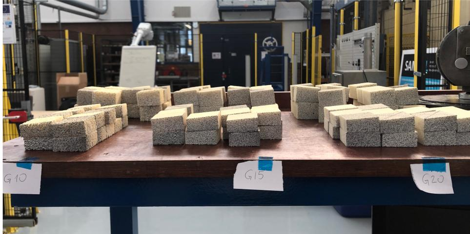
**Figure 5-6:** Polyurethane foam samples prepared for DIC and compression testing.
