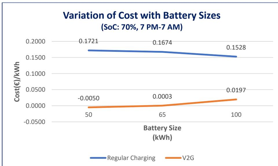
Figure 5.4 Variation of Cost with Battery Sizes
