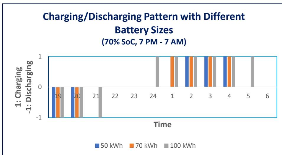
Figure 5.2 Charging/Discharging Pattern, 70 % SoC & 7 PM Arrival, Different Battery Sizes
