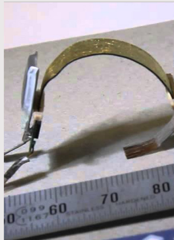
Figure 25 This inchworm robot carries its LiPo battery on its back using IPMCs actuators to move
