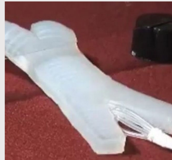
Figure 13 A soft robot with bulbous air muscles that can perform multiple ways of locomotion dependent on which air muscles are compressed
