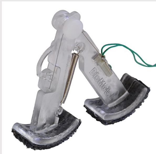
Figure 16 This Nitinol Inchworm moves by contracting an SMA
