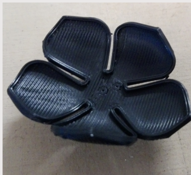
Figure 103 These petals were printed in a different way and each reacted different to heat source they were exposed to
