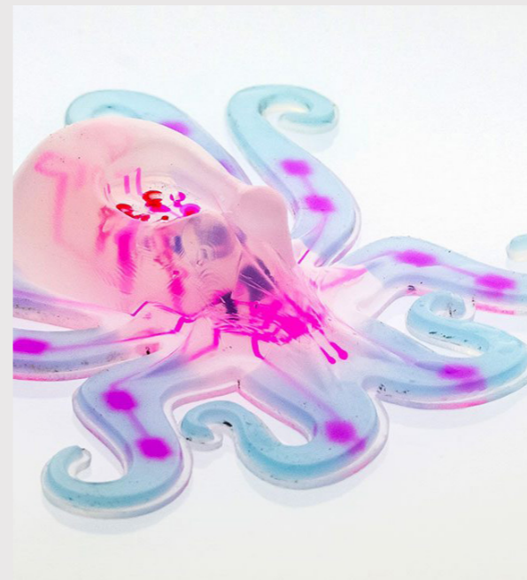
Figure 14 Octobot powered by chemical reactions
