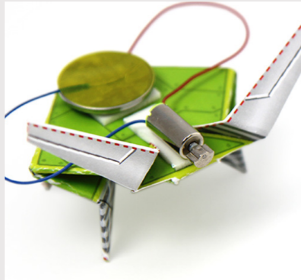
Figure 11 Gamibots are controlled with a rotating motor
