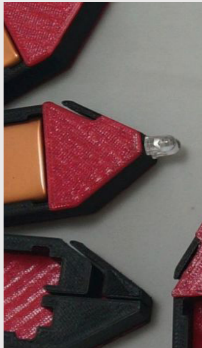
Figure 8 ProtoPasta conductive filament is used to create these flashlights (design by Dustin Cram)
