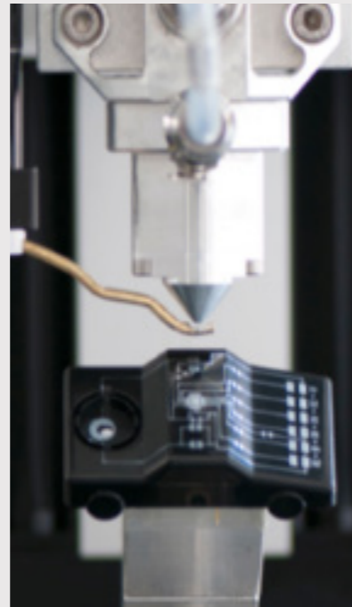
Figure 9 Aerosol Jetting is used to lay down conductive traces by Neotech
