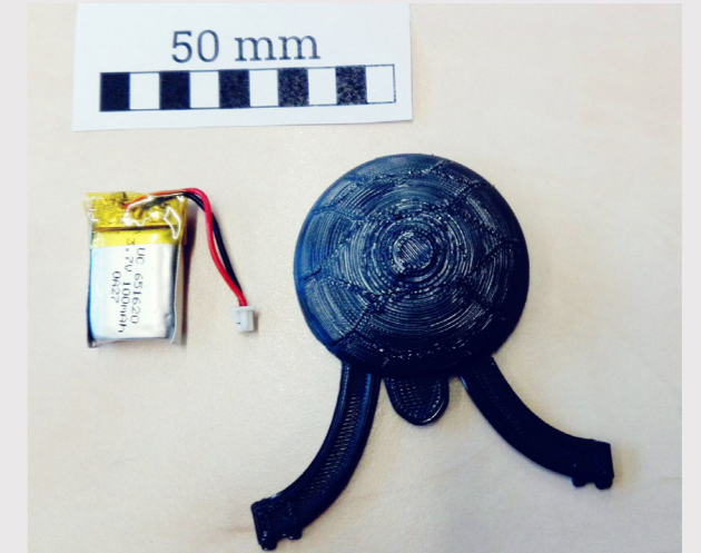
Figure 85 The battery that needs to fit inside the shell of the Turtle Tinybot
