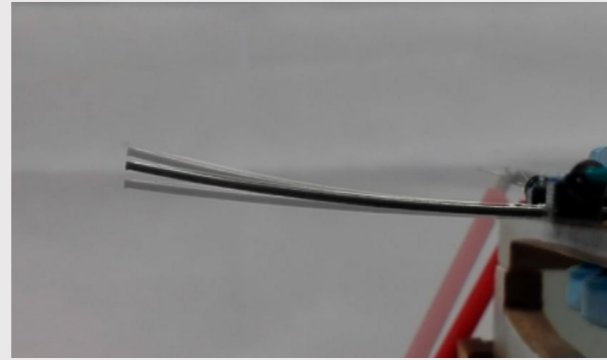
Figure 95 A sample with a heated rim can move up and down. The deflection is however little
