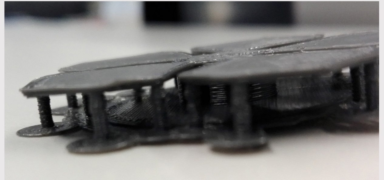
Figure 31 Custom support embedded in the model will ensure gentle removal: columns (Ø1.3 mm) with a brim
