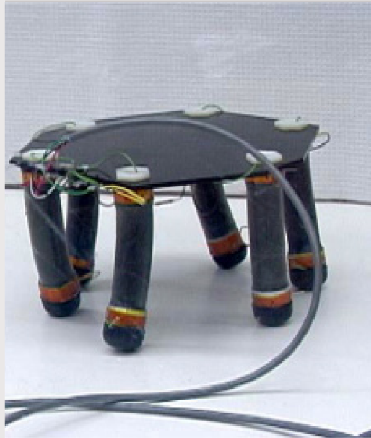
Figure 22 MERbot is able to walk with 6 roll actuators
