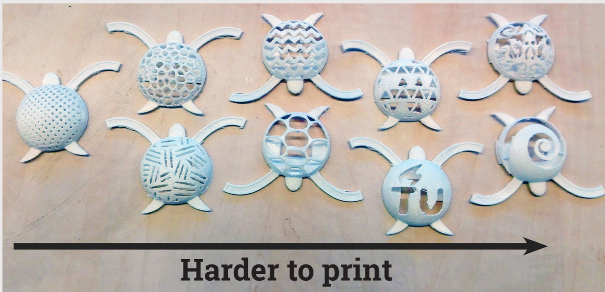
Figure 83 Different iterations placed in order from easy to hard to print
