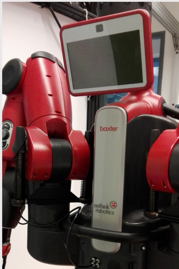
Figure 12 Baxter Robot stationed in Applied Labs at the faculty Industrial Design Engineering
