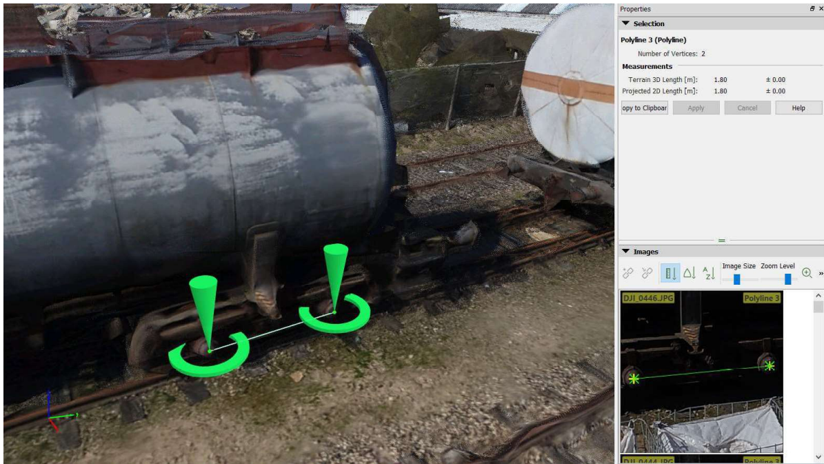
Figure 4.4: Measurement of the wheelbase in the point cloud with an error estimation smaller than 1 centimeter.
