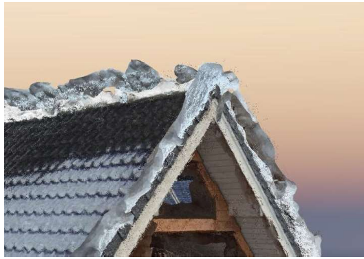
Figure 4.3: Falsly generated points above the rooftop.
