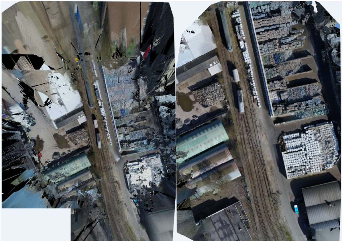
Figure 4.6: Difference in orthomosaic with the raster flight on the right side taken along and not on the left.
