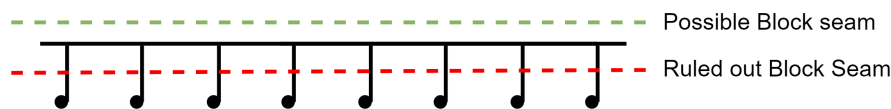
Figure 3.2: Example intersection of a stiffened panel where seams are placed on side without stiffeners
