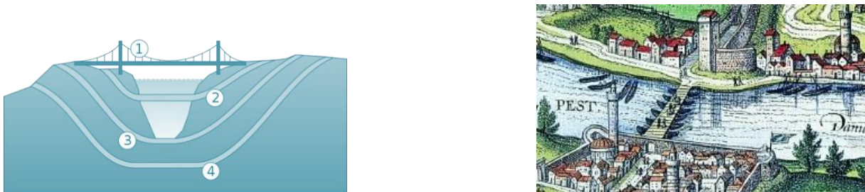
Figure 1: Alternatives for crossing a waterway (a), the application of a floating bridge over the Donau (b)
