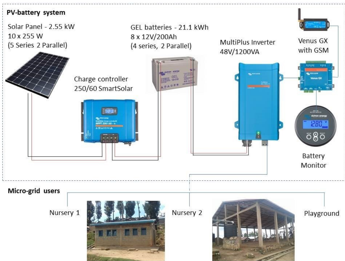
Figure 3: The micro-grid system components in the Kigeme refugee camp (HEED, 2020).
