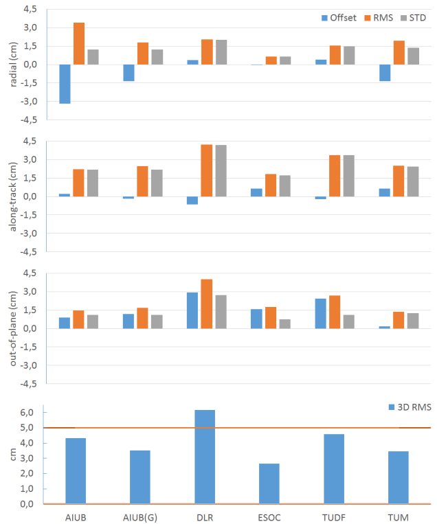
Fig. 2. RSR #1 comparison interval: Mean values (cm) of daily offsets, RMS and standard deviations from comparison between official CPOD orbits and orbits from QWG institutions.
