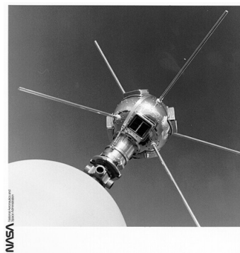
Figure 1.1: An image of the Vanguard 1 satellite with its solar cells in the centre [3].
