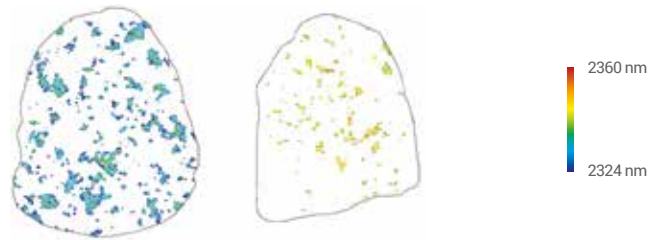
Figure 6.13: Selected examples of maps showing the wavelength position of the chlorite Mg-OH absorption feature. Mapping was only performed on pure chlorite spectra (i.e. no absorption features by any other mineral).
