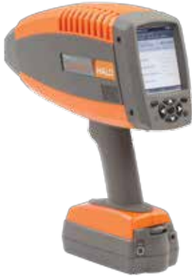
Figure 3.2: Handheld SWIR spectrometer (ASD, 2017).
