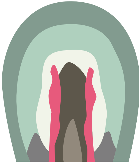
Figure 4.2: Ore mineralisation zones of a generalised porphyry copper deposit (based on Lowell & Guilbert, 1970). Typical dimensions are 1.2 x 2 km horizontally and 3 km vertically. > indicates relative mineral proportions.
