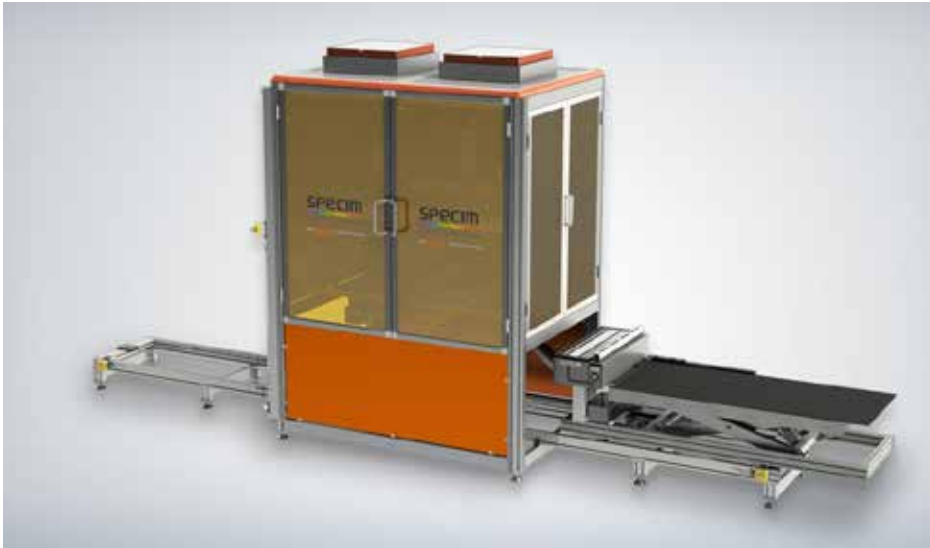
Figure 2.2: SisuRock drill core scanner (SPECIM Ltd., Oulu, Finland). Entire core trays of maximum 1.50 x 0.64 m can be fed through the instrument (Specim, 2017).
