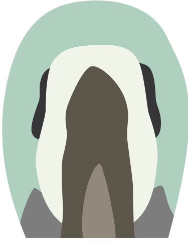
Figure 4.1: Hydrothermal alteration zones of a generalised porphyry copper deposit (based on Lowell & Guilbert, 1970). Typical dimensions are 1.2 x 2 km horizontally and 3 km vertically.
