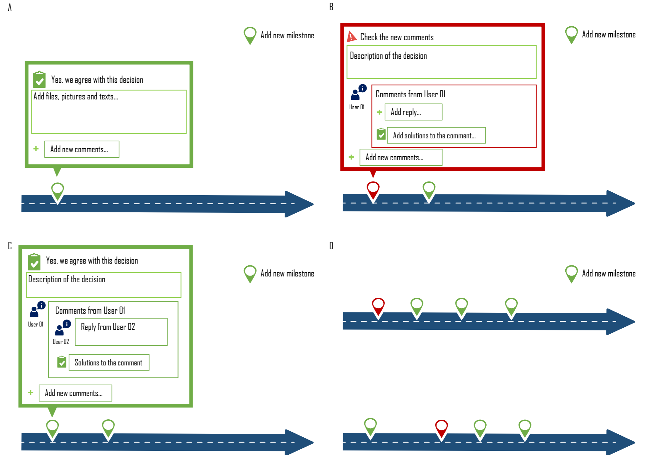
Figure 5.4 Interactive group page of the tool. A: Users can add group decision via the green button “Add new milestone” and add comments to the decision within the “New comments” block. B: Red sign indicates there is a comment needing to be addressed. Users can add response or solutions to the comment and mark the comment solved. C: When the comment is solved, the sign turns green again, while the discussions of the comments are saved on this page for future references. D: The original group page without any expanded signs.
