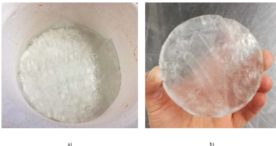
Fig. 10 a) and b) Czech glass cast at 950°C. Post-processing is required to remove the shrinkage of the top surface and reveal the actual transparent glass
