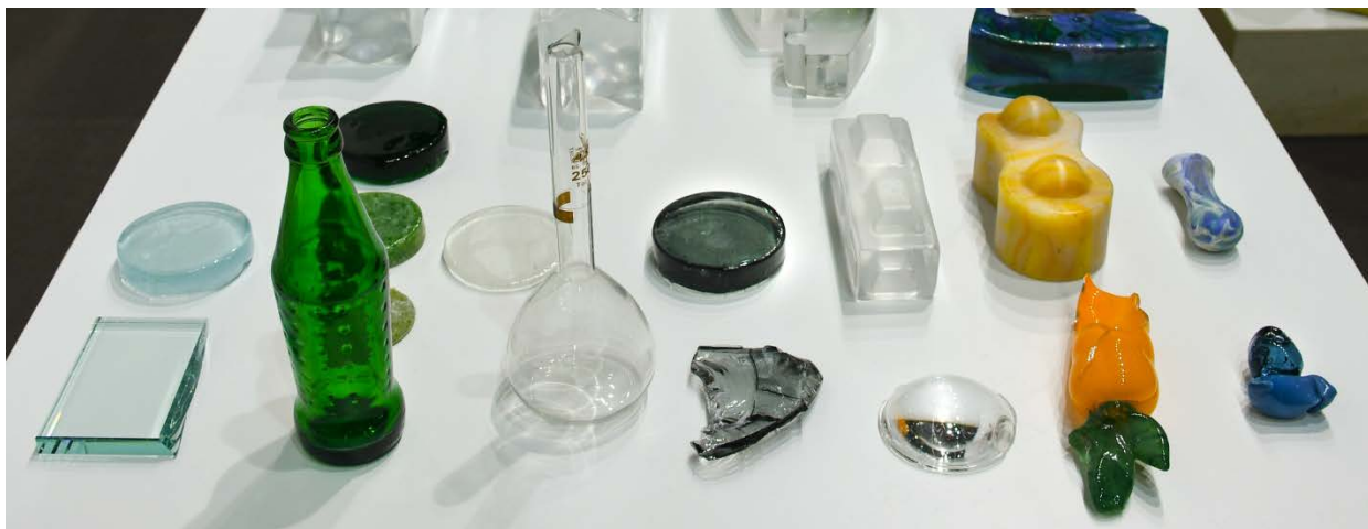
Fig. 21 Successful casting of pieces of (from left to right) float glass, bottle, laboratory tube, computer screen panel, lens, and mouth blown glass, demonstrating the numerous possibilities that arise in creating unique building components.
