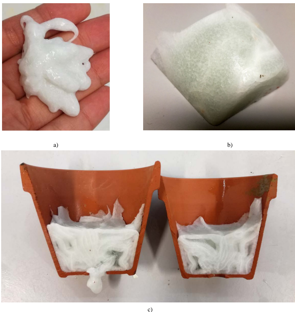
Fig. 16 Results from the kiln-casting of two different types of clear bottles at 970^{\circ}\text{C} . a) Droplets that flowed from the flowerpot down to the mould, b) glass part that fused inside the flowerpot. In this picture, the surface in contact with the flowerpot is seen, c) flowerpot cut in half, showing the layering of the fused glass and the glassy areas within the crystallized mass.
