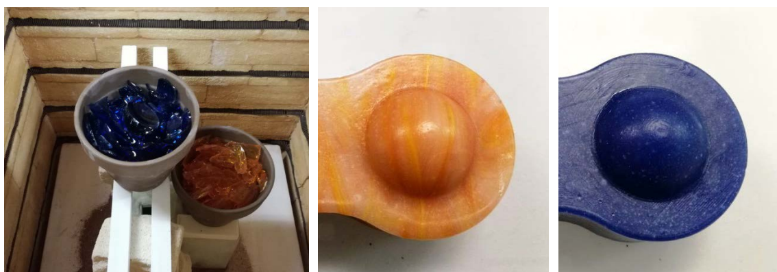
Fig. 6 a) Set-up of the kiln, b), c) glass ceramic samples resulting from the mouth-blown glass waste.
