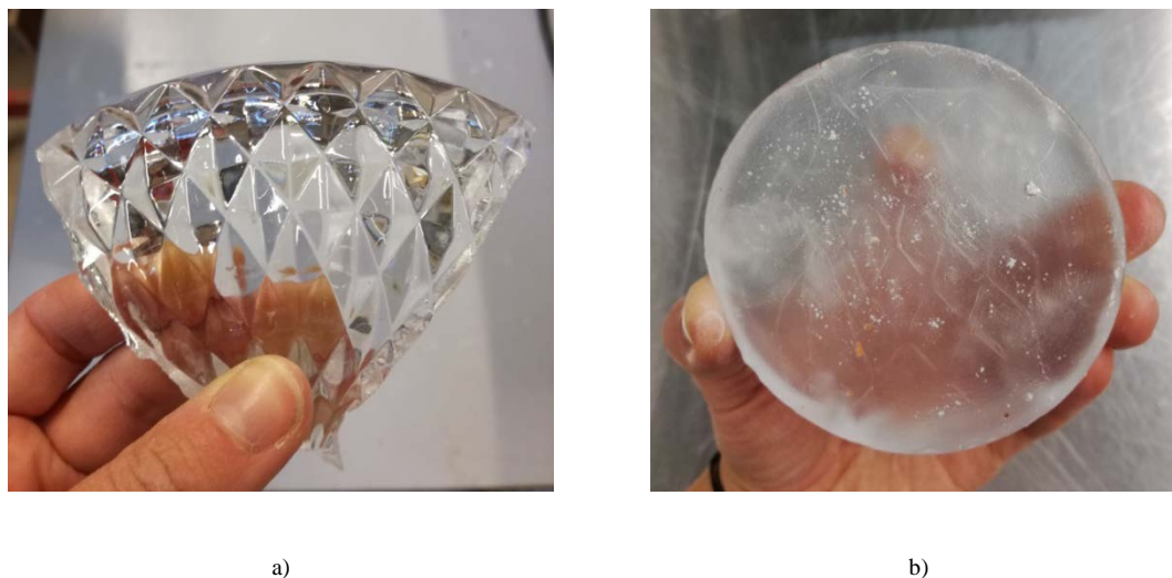
Fig. 11 a) and b) Pressed crystal glass before and after casting at 950^{\circ}\text{C} . The pattern of the glass remained as a trace at the bottom surface of the sample. Upon post-processing, the glass will be transparent.
