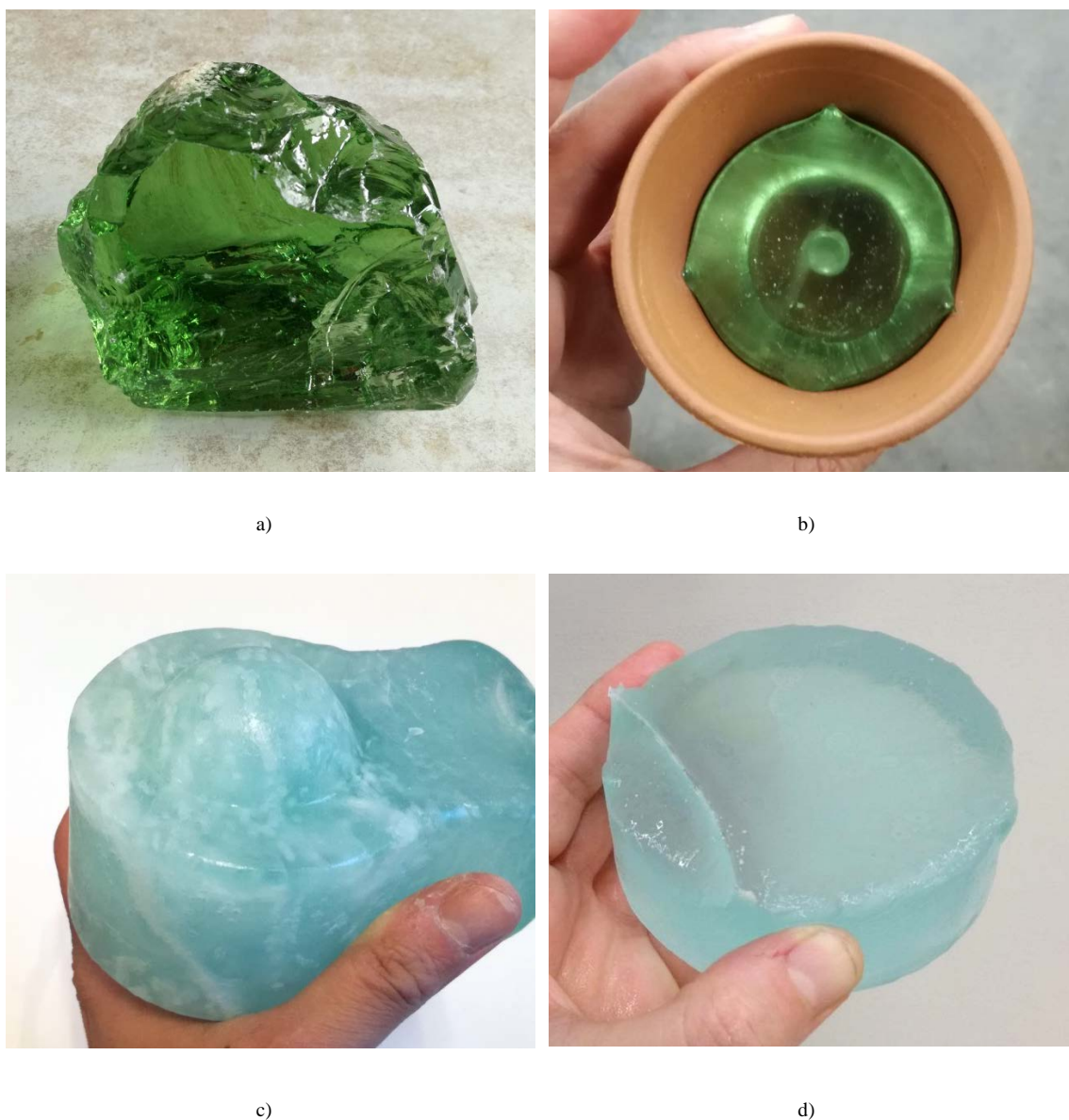
Fig. 9 a), b) PPG furnace waste green glass before and after casting at 860°C, c), d) PPG furnace waste aquamarine cast at 860°C and 1.200°C respectively.
