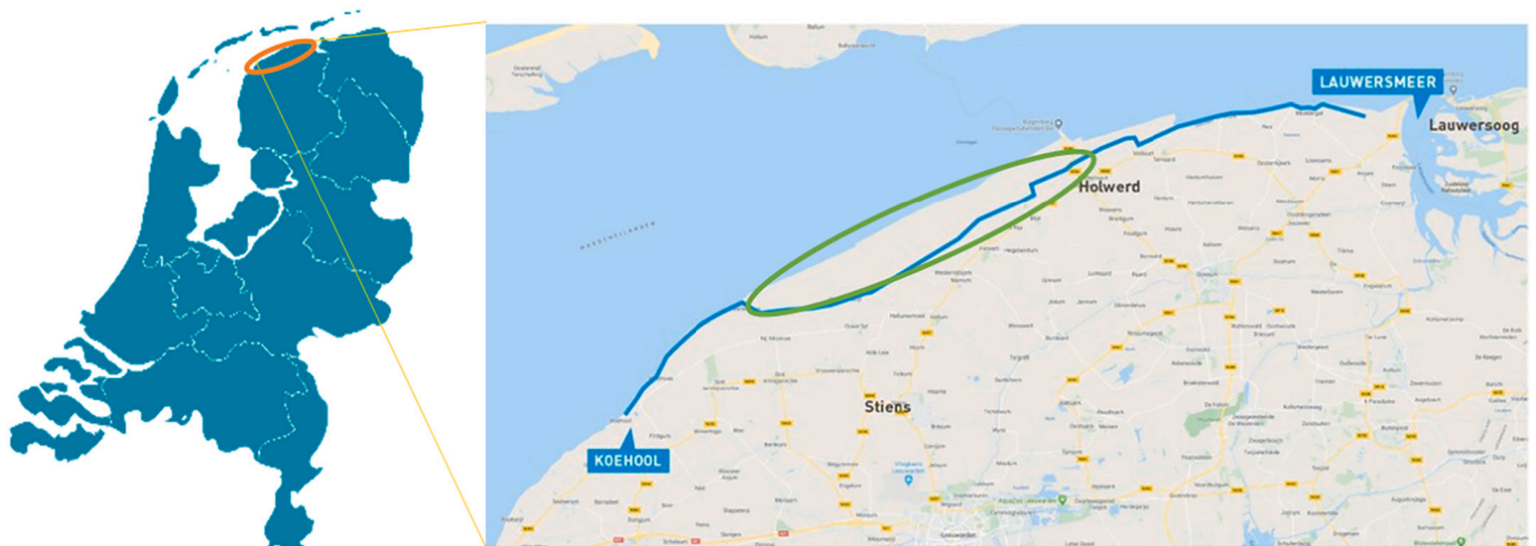
Fig. 2. Location of the study area in the Netherlands and Fryslân. The blue line indicates the dike trajectories along the Frisian coast that will not meet the Dutch flood safety standards over the next 50 years without reinforcement; the green circle indicates the location of the case study site NFB (Adapted from Wetterskip Fryslân, https://www.wetterskipfryslan.nl/projecten/koehool#h2_1; ) (For interpretation of the references to colour in this figure legend, the reader is referred to the web version of this article.)
