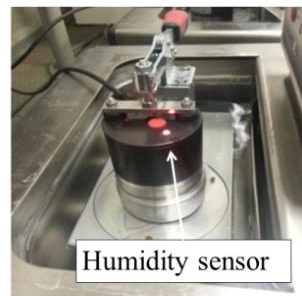
(d) Placing the humidity sensor (with slightly higher temperature (20.3 °C)) on the sample holder
