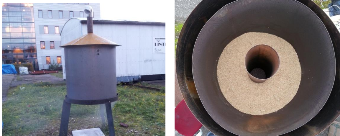
Figure 4.1 The drum incinerator for RHA production, which is similar to the equipment used by Tuan [6].
