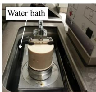
(c) Placing the sample holder in the water bath for at least 0.5 h
