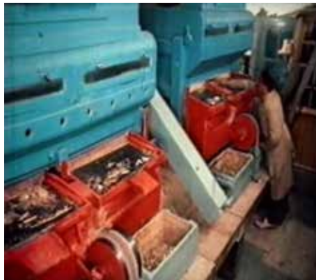
3. The grain is weighed and cleaned before it goes into the silos
