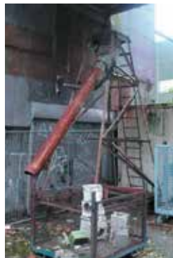
Left behind devices to take the grain from the silos to the workfloor (CV Maassilo. 1951)
