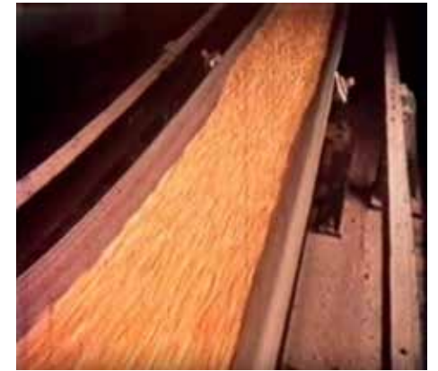
4. At the distribution floor the grain is transported to the tube that goes into the silos
