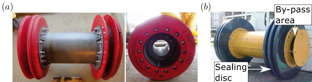
Figure 1.3: (a) By-pass pig with by-pass in the centre (taken from [53]). (b) By-pass pig with a deflector disc (taken from [96]).
