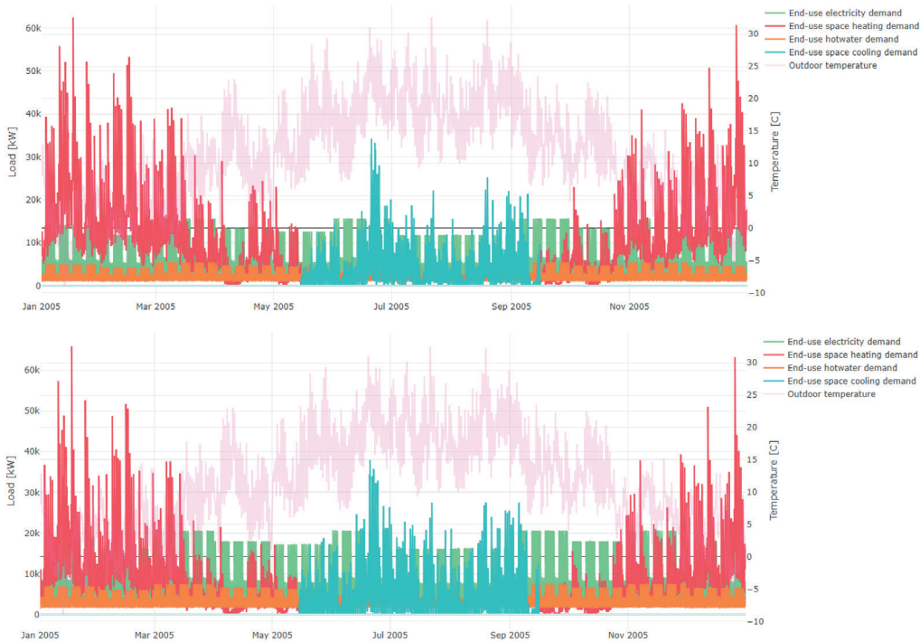
FIG. 3.8 Energy demands in the district and outdoor temperature throughout the year for the Status Quo (top) and Baseline scenario (bottom).
