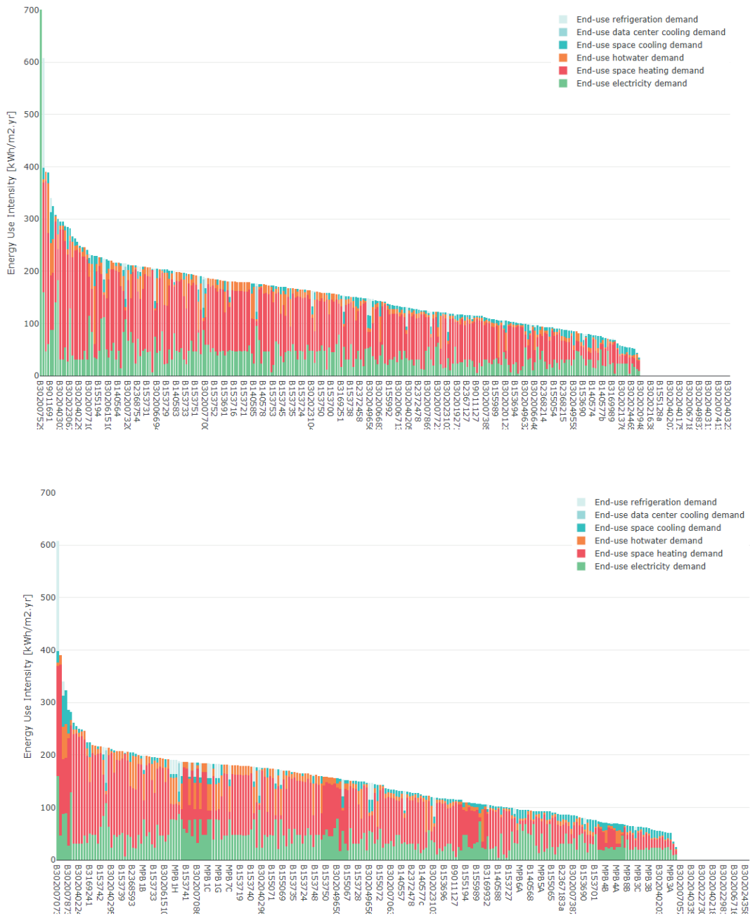
FIG. 3.11 Energy use intensity (kWh/m 2 -yr) for space heating and cooling, domestic hot water and electricity for each building in the Status Quo (top) and Baseline scenario (bottom).
