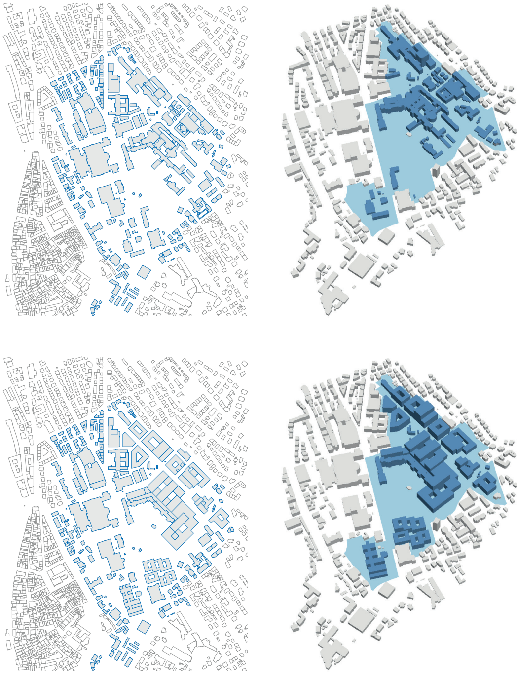
FIG. 3.5 Visualizations of the CEA model for the Status Quo (top) and Baseline (bottom), orthographic (left) and perspective (right).
