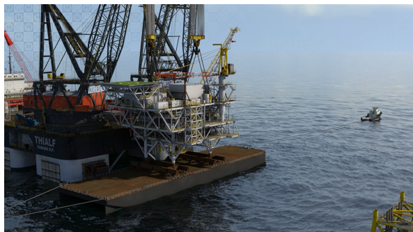
Figure 1.2: Load transfer phase
