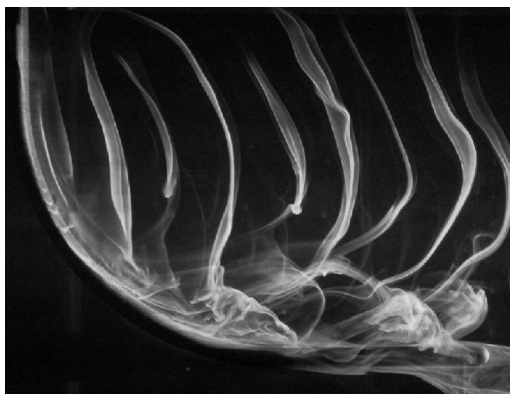
Figure 2.15: Flow visualization for a curved cylinder in uniform flow parallel to the plane of curvature Re = 100 [Miliou et al., 2003]
