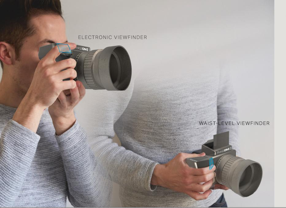
Although its iconic image, medium format cameras are perceived as rather big and bulky. That is predominantly caused by a traditional optical system (single-lens reflex) and the larger light sensitive element (digital sensor or film negative). Due to advancing sensor technologies, it becomes possible to capture an image without the mirror reflex for larger sensors (with an acceptable latency).
