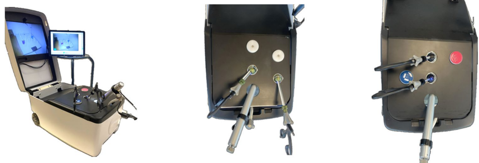
Fig. 2 Left: a picture of the setup featuring the box trainer, newly designed panel, the newly located screen and two Maryland graspers. Middle: a picture of the designed panel with the trocars and camera in triangular configuration. Right: a picture of the designed panel with the trocars and camera in the midline
