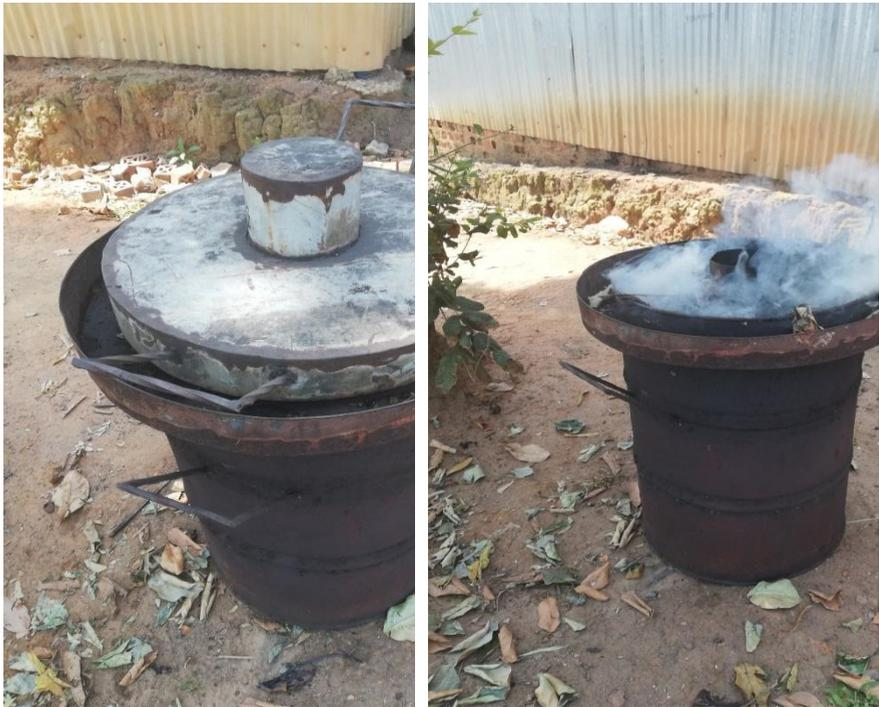
Figure 26. Photo of biochar carbonization
