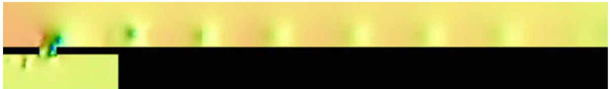
Figure 2.23: Vortex transport due to a M_0 = 0.3 grazing flow, instantaneous density field, image adapted from Tam et al. [47].
