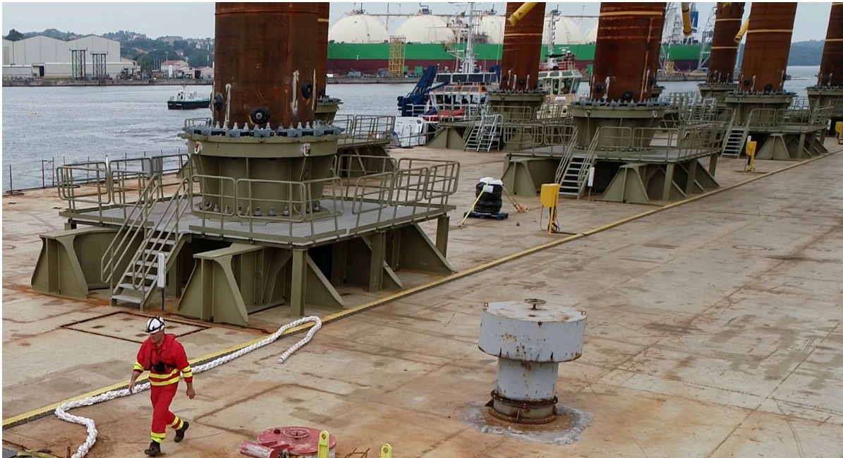
Figure 1.8: Close up of sea fastening structures designed for the transport of jacket structures, taken from [18]
