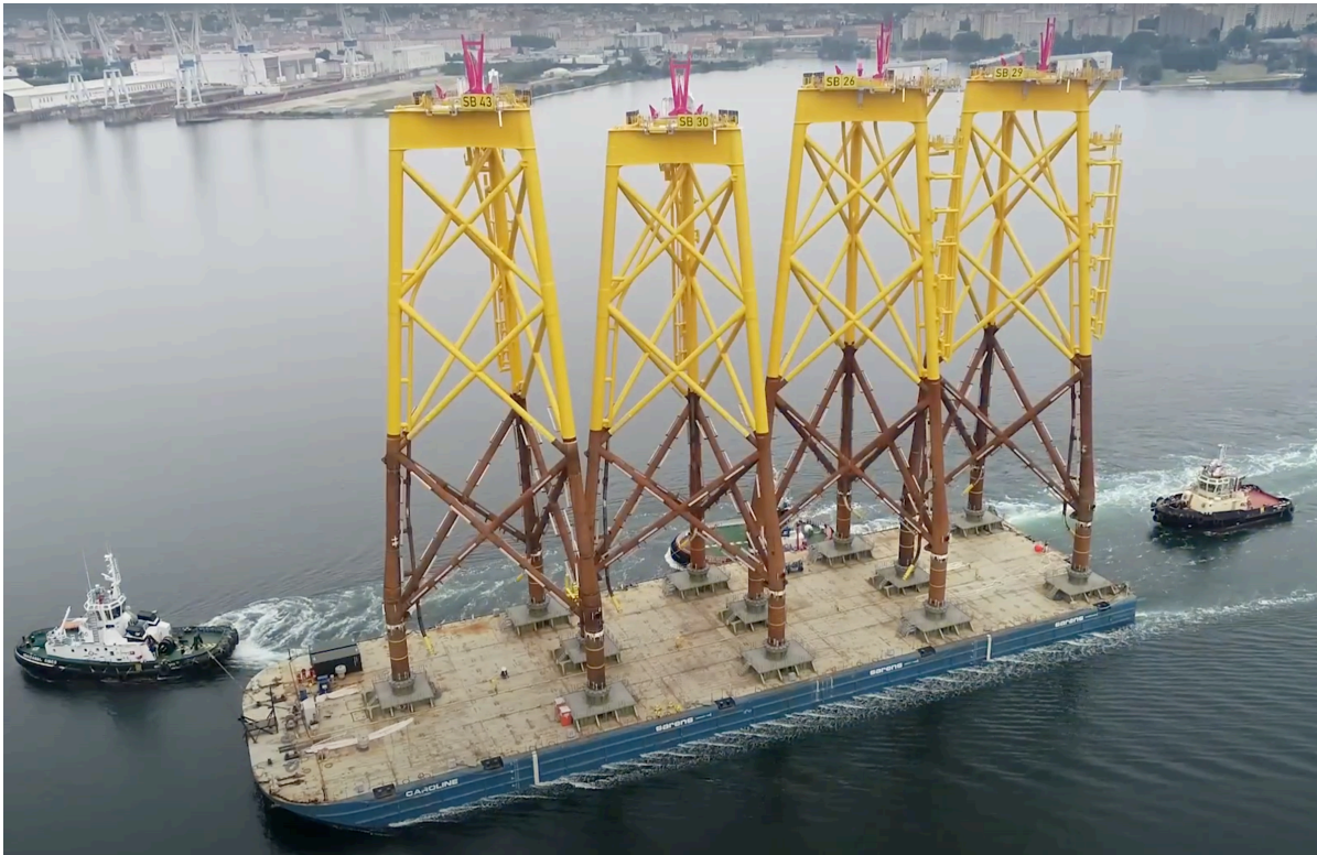
Figure 1.7: Picture of jacket support structures which are sea fastened to a transport barge during transport, taken from [22]
