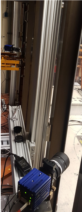
Figure C.3: sCMOS cameras set-up outside the wind tunnel walls
