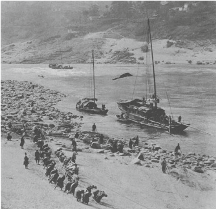
Fig. 2 Image of trackers from Worcester (1971); page 5 entitled 'Hauling a junk over the Yeh T'an. The extra tracking hawser can be seen, as can the sampan which supports the bamboo rope; released under a Creative Commons Attribution-NonCommercial-NoDerivatives 4.0 International Licence'
