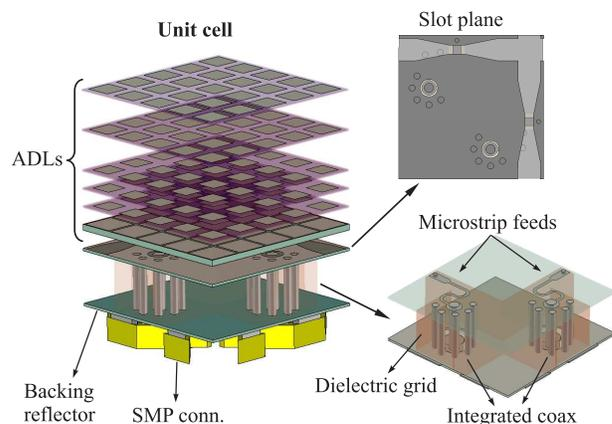
Fig. 2. Three-dimensional view of the final unit cell.
