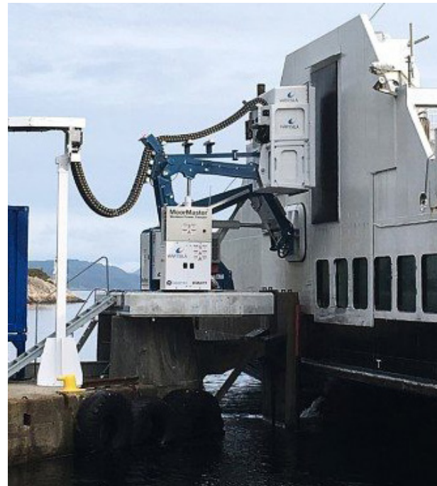
Fig 33. Wartsila Induction Charging (Sorfonn, 2016)
