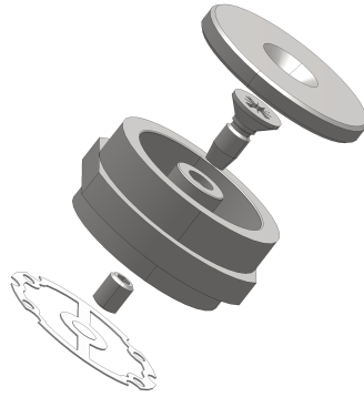
Figure 1.2: Exploded view of the load cell designed by Intralox.
