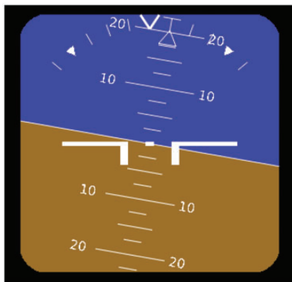
Figure 1. The moving-horizon type AI indicating an aircraft turning to the left, tilting the horizon to the right. The aircraft symbol (white wings) remains static in the center of the display; the horizon rotates and moves up with the aircraft roll and pitch angles, respectively. The figure shows the display format used in the experiment, which is a simplified version of the AI used in large jet airliners.
