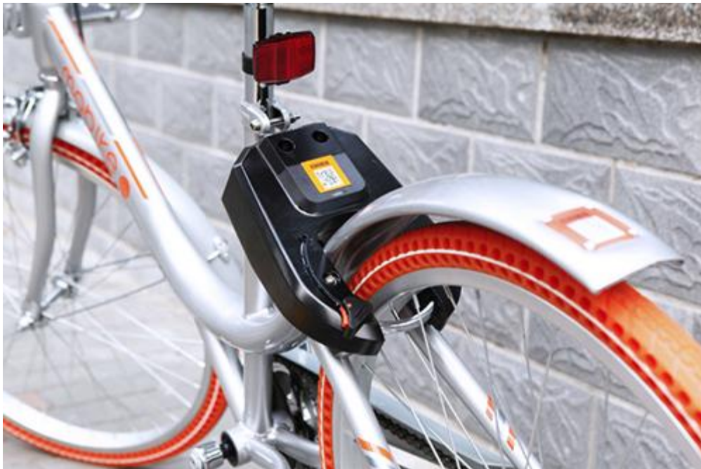
Figure 2.1. Mobike's smart lock (E-stronger., 2017)
