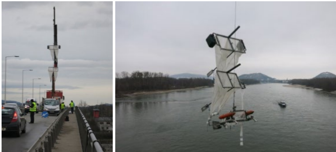
Figure 5: Three-layered net for suspended litter collection, deployed from a crane (Hohenblum et al., 2015).
