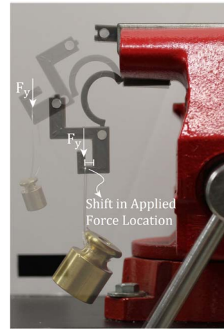
Fig. 18 Illustration of the original location of the applied force at the tip of the folding CM and its shift caused by the increase in weight
