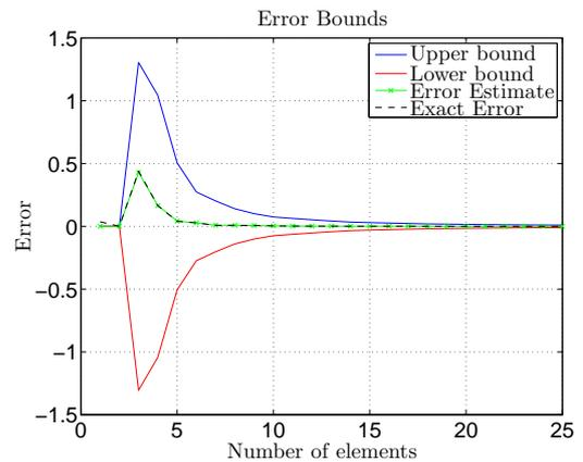
(b) Error bounds for the case  $*d * d\phi_2^0 = f_2^0$ .**Figure 4.7:** Convergence of the effectivity index and the error bounds for the case  $*d * d\phi_2^0 = f_2^0$ .
