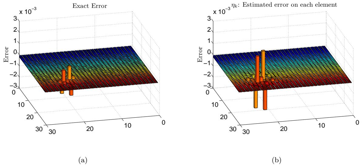
**Figure 4.36:** Exact and estimated error over each element for 900 elements.
