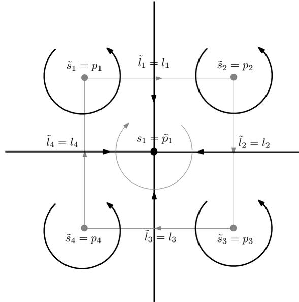
**Figure 2.4:** Primal cell complex in grey and dual cell complex in black.
