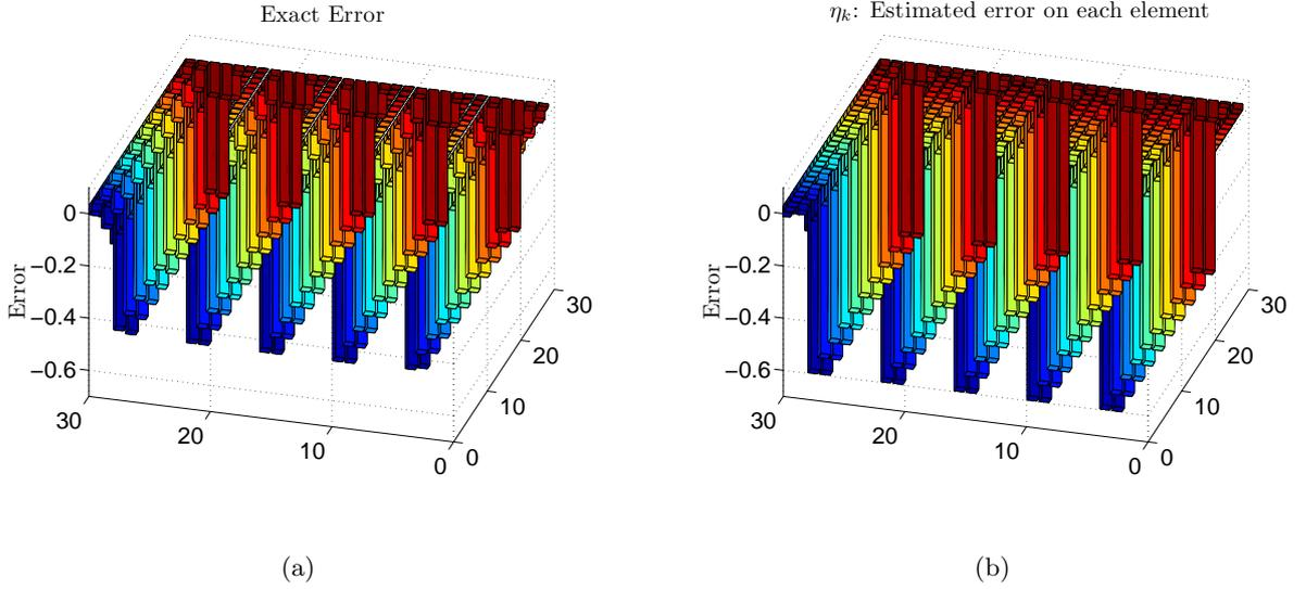
**Figure 4.28:** Exact and estimated error over each element for 900 elements.
