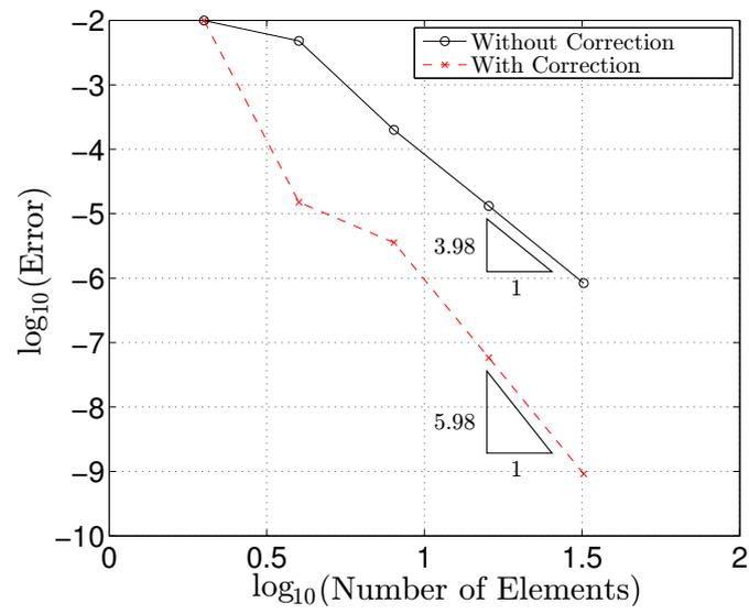
**Figure 5.1:** Error in the target functional with and without correction.
