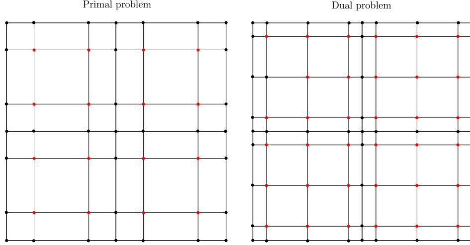
**Figure 4.24:** Gauss-Lobatto grids used for solving the primal and the dual problems.
