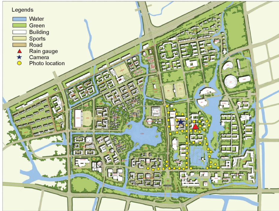
Fig. 5. Locations of the sensors (smart phones and cameras) used to collect rainfall images.
