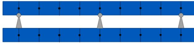
Fig. A.1. Vessel, cargo and sea-fastening system for cargo with equal length to the vessel length. The cargo is connected using a pinned condition at  $0L$ ,  $0.5L$  and  $L$ .
