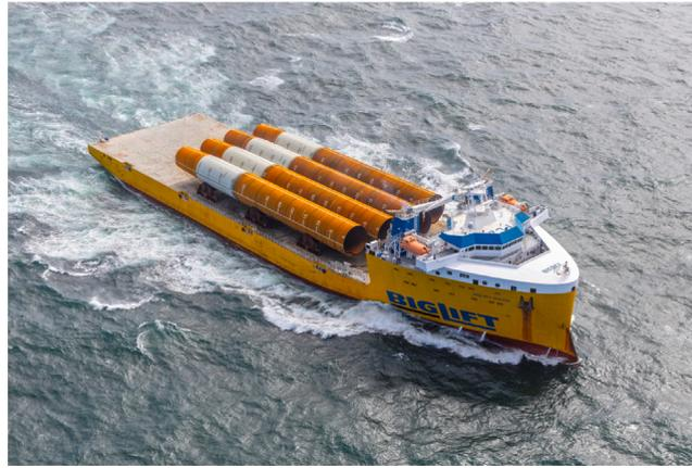
Fig. 2. Base case MC-class heavy-lift vessel transporting monopiles.
