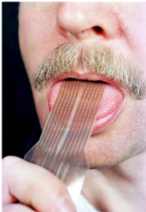
image / figure 2: Tongue Display Unit (TDU) for "high definition electrostatic spatial information" (Kaczmarek, 2010)
