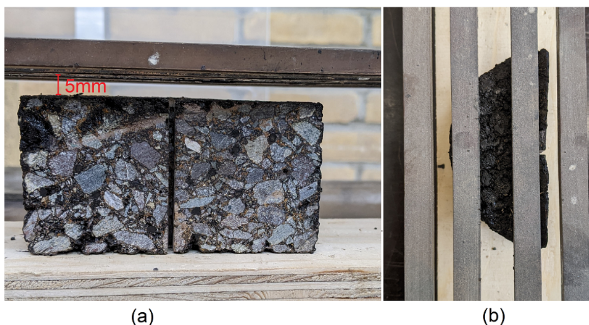
Figure 4.4: An SCB sample under induction coil from a) front view and b) top view.
