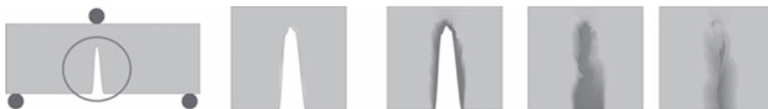
Figure 2.14: Schematic of the basic principle of self-healing materials, with reaction progression from left to right. Mechanical load induces a crack, resulting in activation of a mobile phase. The mobile phase closes the crack and is immobilised post healing event. [38]
