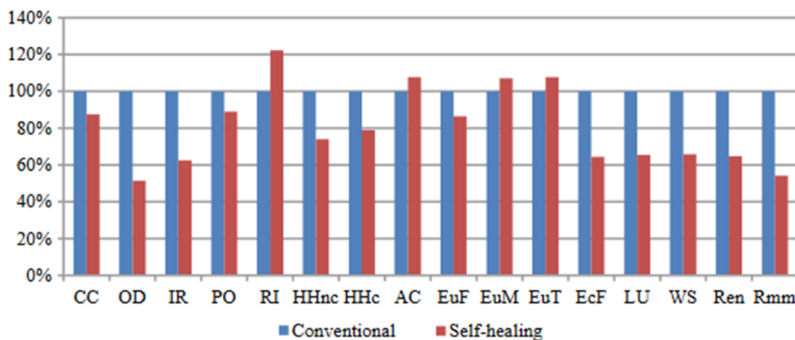
Figure 2.26: Comparative LCA study of self-healing asphalt vs conventional mix. The environmental impact categories covered in the study are listed as follows: Climate change (CC), Ozone depletion (OD), Ionising radiation (IR), photochemical ozone formation (PO), respiratory inorganics (RI), human toxicity (cancer (HTc) and non-cancer effects (HTnc)), acidification (AC), eutrophication (terrestrial (EuT), fresh water (EuF) and marine (EuM)), freshwater eco toxicity (EcF), land use (LU), water scarcity (WS), resource use, energy carriers (Ren), and resource use, minerals and fossils (Rmm) [62].
