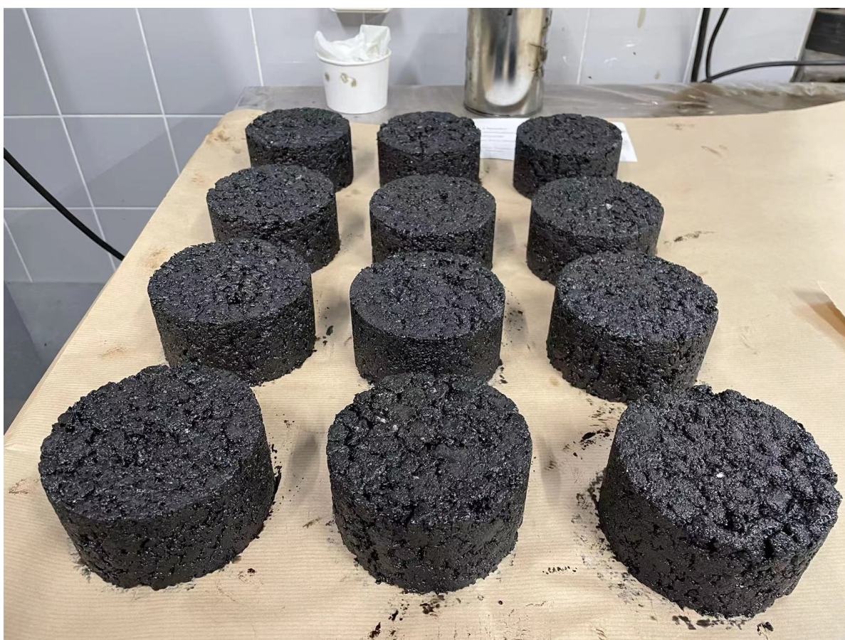
Figure 3.4: 100mm x 50mm samples post compaction
