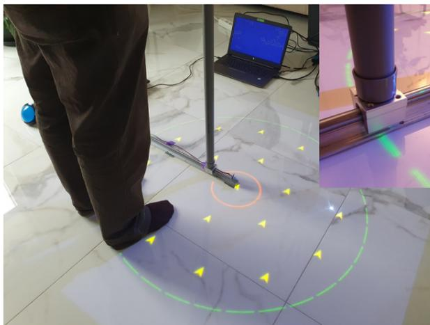
Figure 65: Linear slider with bearing block and a close-up of the bearing block
