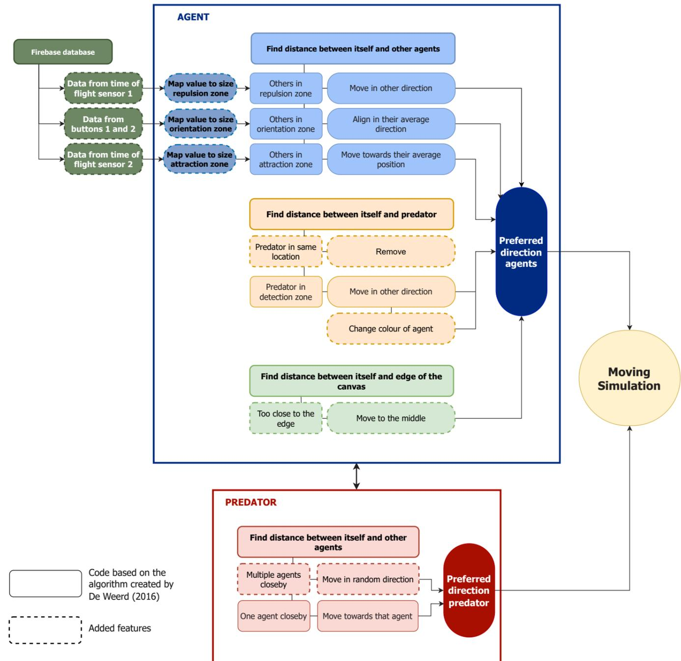
Figure 58: Overview of the script used for the simulation of the moving group. The blocks outlined with a continuous line are code based on the algorithm created by De Weerd (2016). Blocks outlined with a dashed line are added features to the script.
