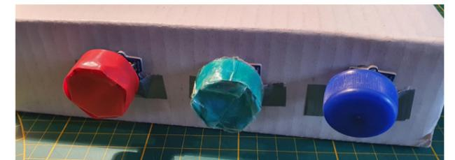
Figure 29: Rotary buttons to adjust the size of the zones
