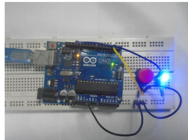
Figure 15: Arduino project with a button and LED (Aqib, 2018)
