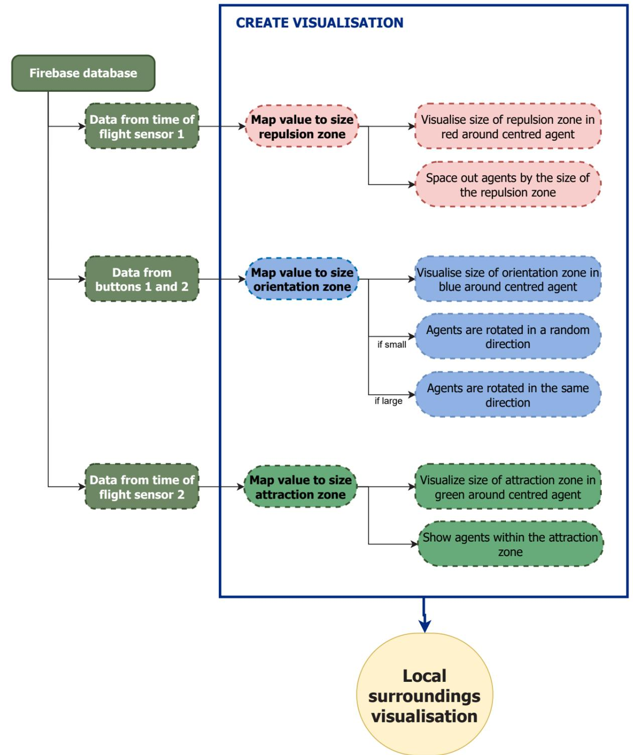
Figure 63: Overview of the script used for the visualisation of the local surroundings around an individual.
