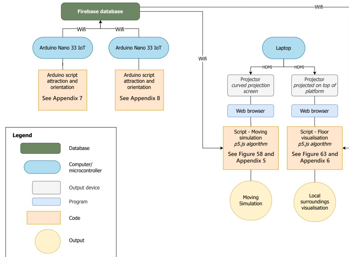
Figure 70: Overview of the communication between the Arduino boards and the two visualisation algorithms.
