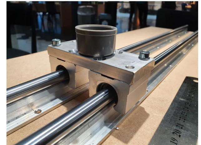
Figure 67: Using two rails and connecting the blocks
