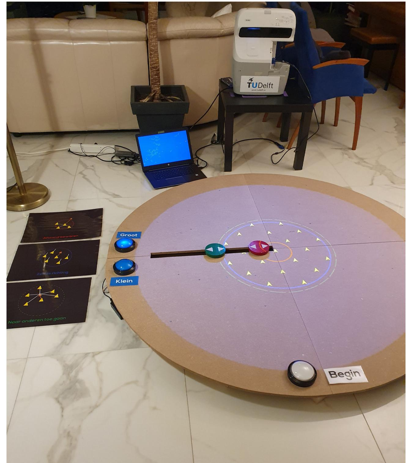
Figure 76: Prototype that is used for the validation in Naturalis. The two disks to move the sliding mechanism are painted in the colour of the corresponding circle, to let the user know which disk corresponds to which circle. Arrows are added on top to give users the use-cue that they are movable. The buttons are annotated with the words 'small' and 'large' for orientation and 'restart' for the restart button.
