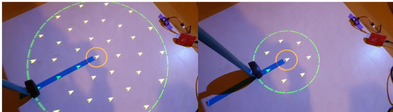
Figure 50: Operational prototype: move handle back and forth and see circles change size accordingly
