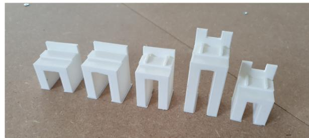
Figure 73: Several 3D printed iterations to find the right design for the time of flight sensor
