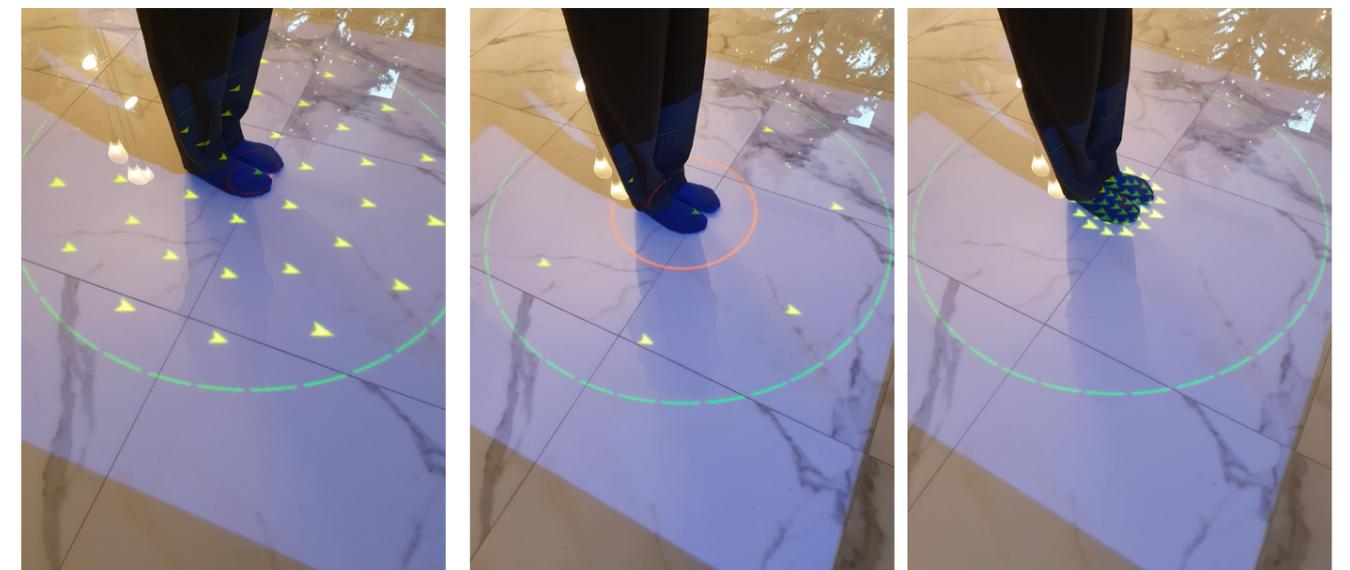
Figure 48: Projection on the floor of 1.5m by 1.5m, with a user standing in the middle. Different sizes of the repulsion zone are shown.
