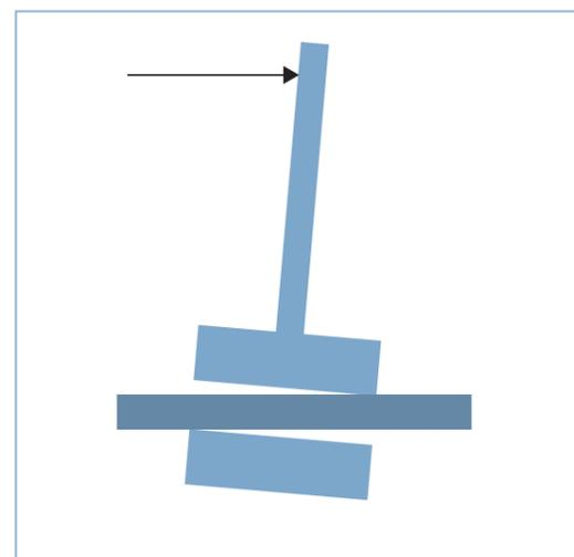
Figure 66: By pushing at a high height, the torque makes the block tilt and create friction
