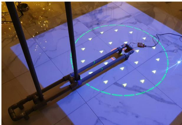
Figure 64: Finding the right dimensions with a prototype made out of PVC tubes and two T-pieces that could slide back and forth.
