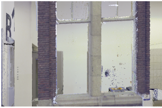
(a) The points visible in the window are reflected points that the laser registered
