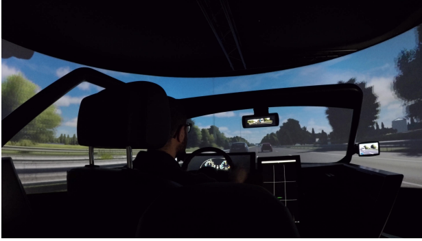
Figure 4: A lane change maneuver during the experiment in the highway scenario on the 6 DoF motion-based simulator
