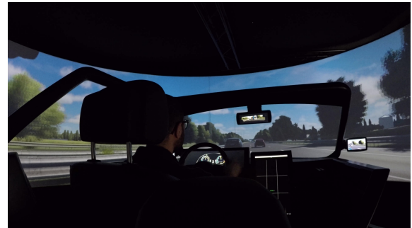
Figure 1-8: A lane change maneuver during an experiment in the highway scenario of the 6 DoF motion-based simulator
