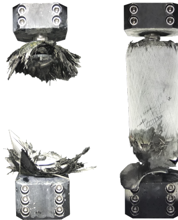
Figure 3.1: Examples of a safe global failure (left) and unsafe dome blowout (right)
