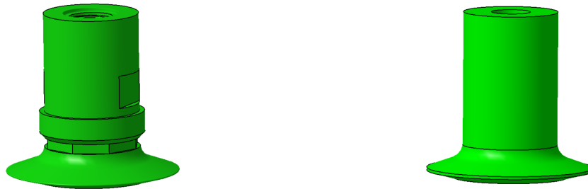
(a) Original geometry of the boss, with threads inside (b) Simplified geometry of the boss, without threads and cutouts
