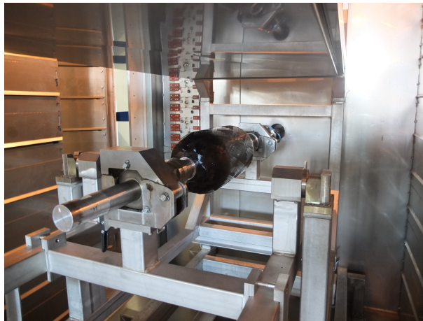
(a) Vessel in curing oven with rotating fixture
