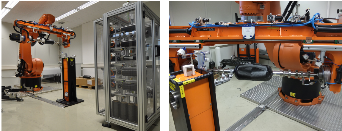
(a) Filament winding setup consisting of the robot with traverse (left), stationary eyelet (center) and creel cabinet (right) (b) Robotic filament winder manufacturing a helical layer, with moving traverse
