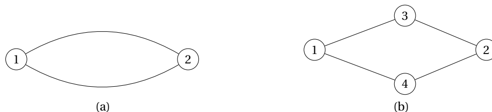
Figure 6.2: Two simple synchmodal transport networks transporting containers between node 1 and node 2. Network (b) has more infrastructure elements (nodes 3 and 4) than network (a). For network (a) 2 challenges have to occur or 100% of the infrastructure elements have to be removed to disconnect the network. For network (b) either 2, 3 or 4 challenges need to occur or either 33%, 50% or 67% of the infrastructure elements have to be removed to disconnect the network.
