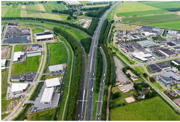
Figure 4.7: Road intersection Gouwe, exchange of vehicles is not possible between all directions [76].
