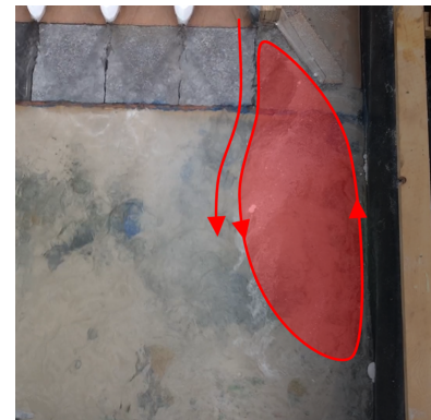
Figure 2.12: Sketch of the horizontal flow pattern observed by BAM Infra at the Afsluitdijk model tests (Top view), adapted from Level (2018).
