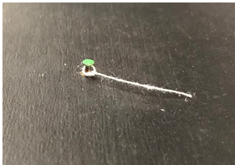
Figure 5.3: Close-up picture of the final tuft design.
