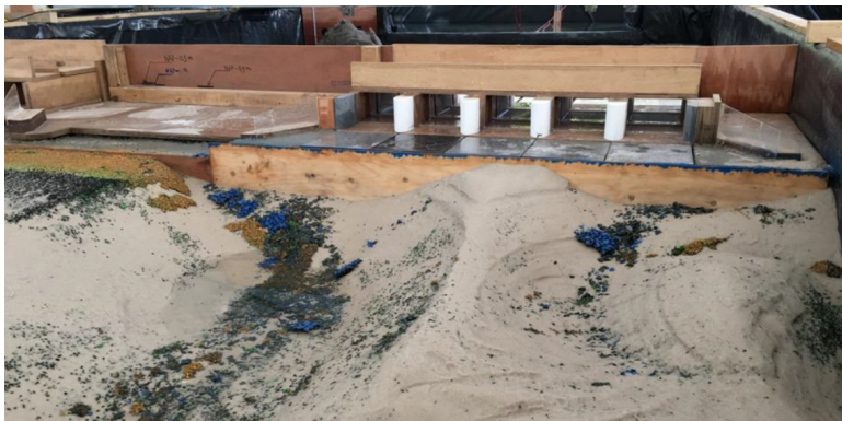
Figure 2.11: Bed topography observed by BAM Infra at the Afsluitdijk model tests (Level, 2018).
