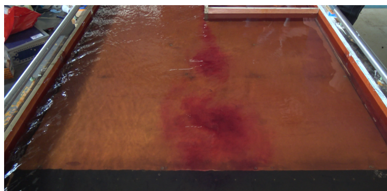
Figure 6.14: The presence of coherent turbulence structures in the mixing layer visualised by dye.
