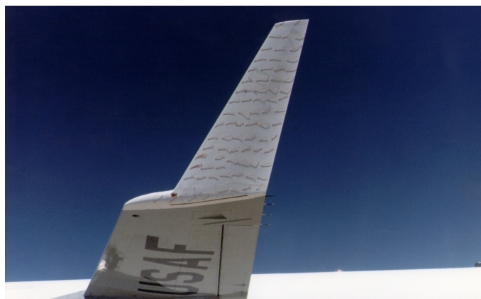
Figure 5.1: Tuft airflow visualisation on an aeroplane winglet by NASA (1979).
