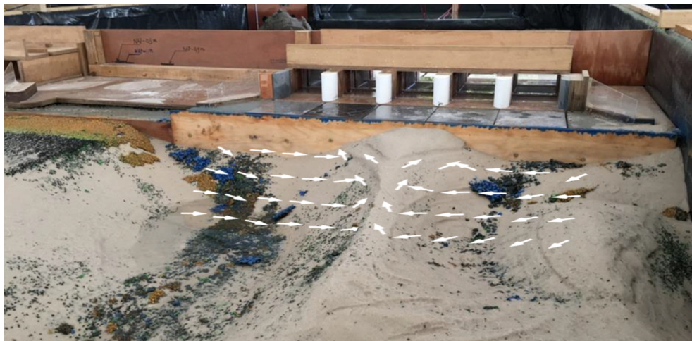
Figure 7.3: Near-bed flow directions of Test 1.3 (left) and Test 1.2.B (right) in comparison to the scour hole at the Afsluitdijk model tests. The white arrows show the time-averaged flow directions. Table 7.2 provides the specifics of the tests that are compared. Please note that the flow directions were measured in configurations that differ from the Afsluitdijk configuration. Subsequently, this figure is not just a first indication of the near-bed flow directions during the Afsluitdijk tests.
