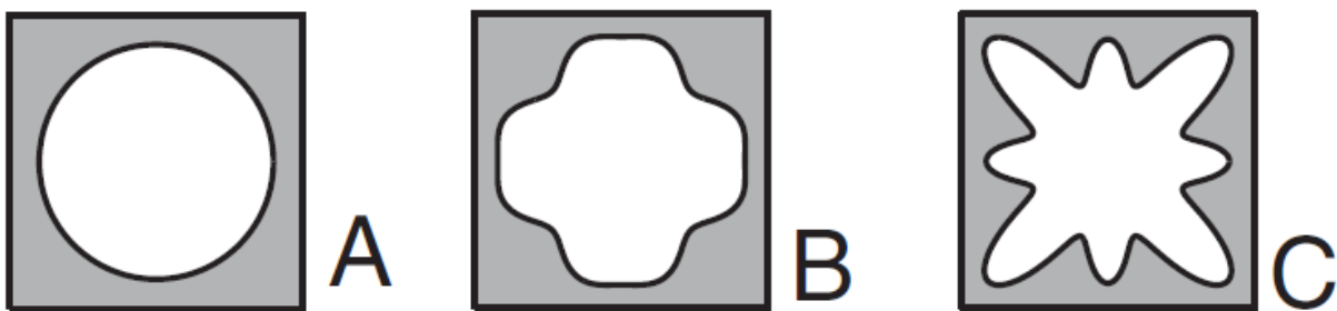
Figure 1.36: Pore shapes used to investigate their effect on auxetic behaviour, image adapted from ref. [96].
