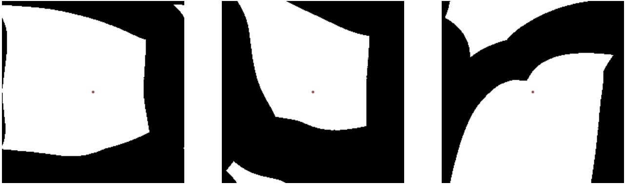
Figure 2.1: Examples of microstructures produced by the Voronoi diagram growth-based method. Black pixels represent material and white pixels represent void.
